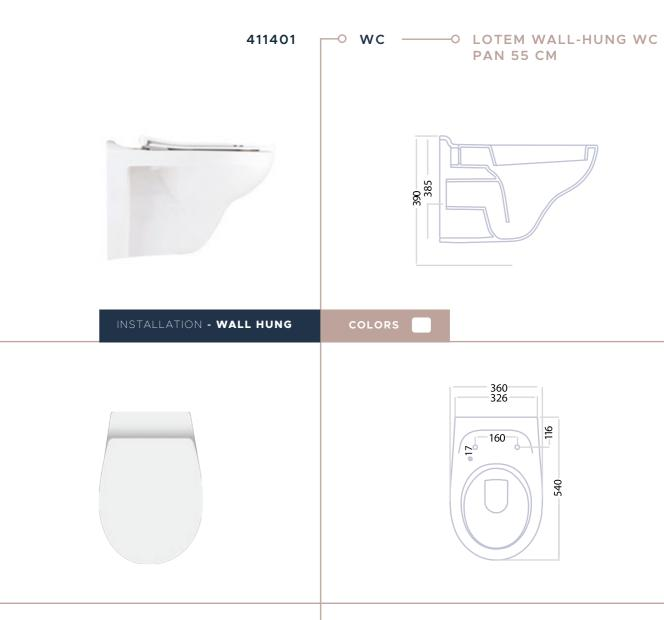
Wall hung wc with rounded front edges and a conformation of recesses that gives particularity to the product. It is compatible with concealed cistern.
