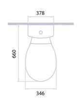
Close-coupled wc with a rectangular water tank. Can be installed with wall or floor drain. Made with a special antibacterial enamel, the monobloc wc can be equipped with an antibacterial seat and a cover board for greater hygiene.
